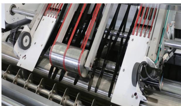
Equipped with servo driven top sheet meeting base sheet, the servo drive helps to deliver a square and accurate feeding for the top sheet and smoothing the feeding.
