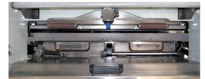
Automatic die cutting frame & plate locking system
